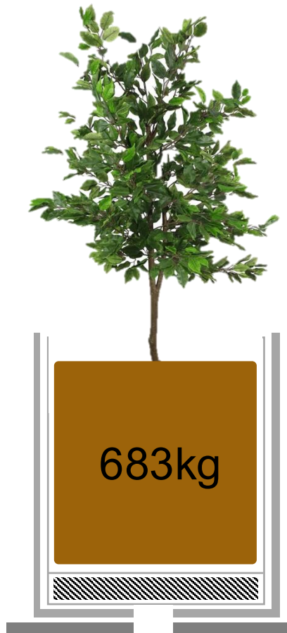
Glass Reinforced Concrete (GRC) Standard Lightweight planter mix 800mm D x 800mm H
